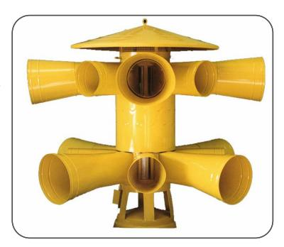
Our most affordable dual tone siren, the 10V2T is designed to excel in almost any application. It's staged horn projectors provide a large, even coverage area. Rated at 122 dB at 100 feet, the Model 10V2T is an OMNI-DIRECTIONAL siren which produces continuous 360° coverage, a clear advantage over rotating sirens.
