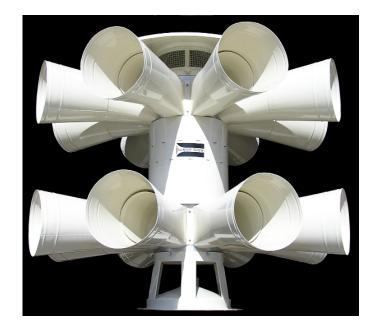
Large enough to tackle almost any application, the Sentry Model 20V2T is at the top of its class. Taking advantage of a continuous duty industrial motor and rated at 124 dB at 100 feet, the 20V2T is an OMNI-DIRECTIONAL siren which produces continuous 360° coverage, making it a superior alternative to a rotating or directional beam type siren.
