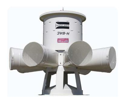
Designed for small towns or Volunteer Fire Departments, the 3V8-H combines large siren functions with cost effectiveness. Utilizing the same effective design and construction as its brother the 3V8, the 3V8-H uses projectors to distribute and organize sound. Rated at 109 dB at 100 feet, the Model 3V8-H is an OMNI-DIREC-TIONAL siren which produces continuous 360° coverage.
