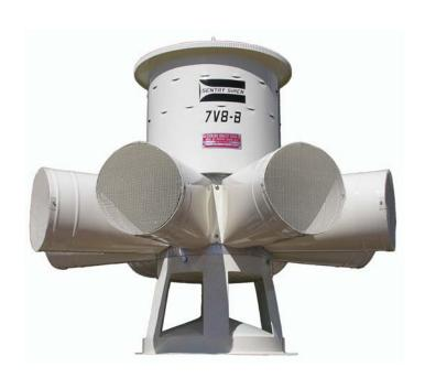
Employing carefully designed horns to project sound over long distances, the 7V8-B is Sentry's newest model. The Model 7V8-B is rated at 118 dB at 100 feet, and like all Sentry weather warning sirens, is OMNI-DIRECTIONAL.
